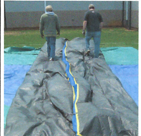
Step 2-6: Fold the Inflatable in 2-3 feet lengthwise & walk out air towards Ports (Blower tubes).
